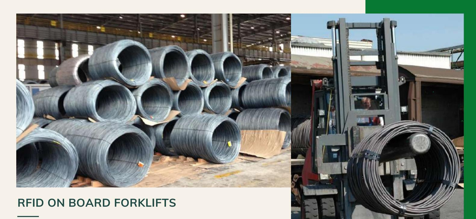
Onboard the forklift there is an antenna able to automatically extract the information on the tags and indicate to the operator the position where to take the coils.
