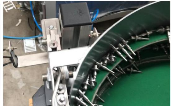
Fig. 8, 9 – Metallic support, machine for metallic support, stud dispenser
